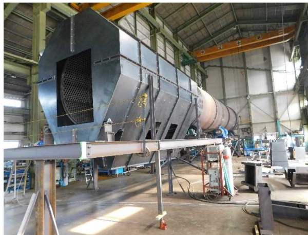
High-efficiency drum-type sorter installation work status
