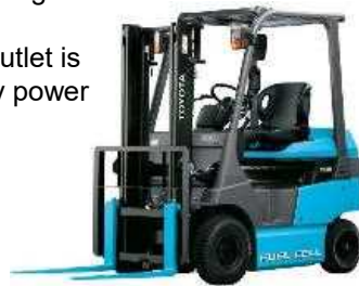
2.5 ton product fuel cell forklift
