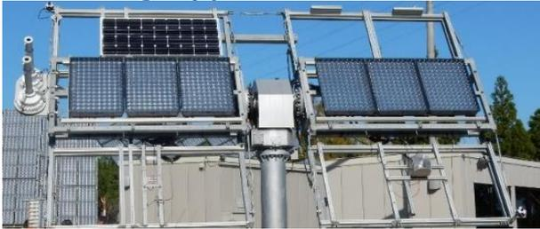
※PV panel with condenser lens. Movable frame keeps optimized angle with solar irradiance (Built at University of Miyazaki )
