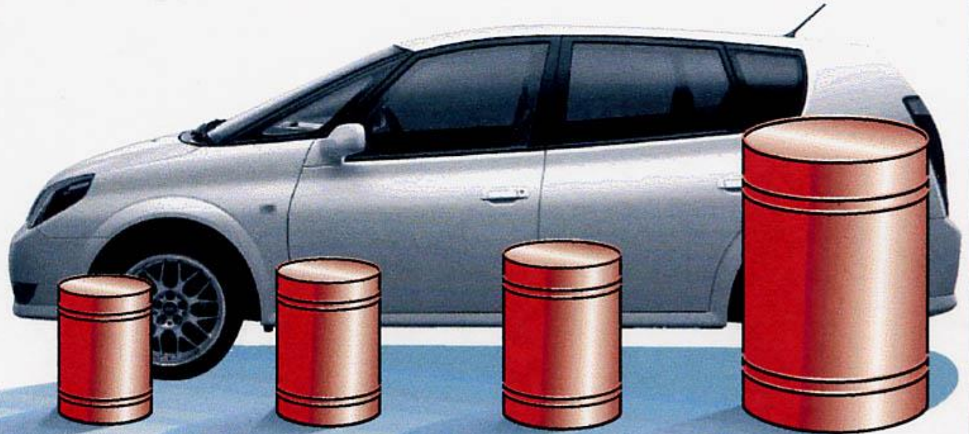
Figure 1 Volume of 4 kg of hydrogen compacted in different ways, with size relative to the size of a car. (Image of car courtesy of Toyota press information, 33rd Tokyo Motor Show, 1999.)
